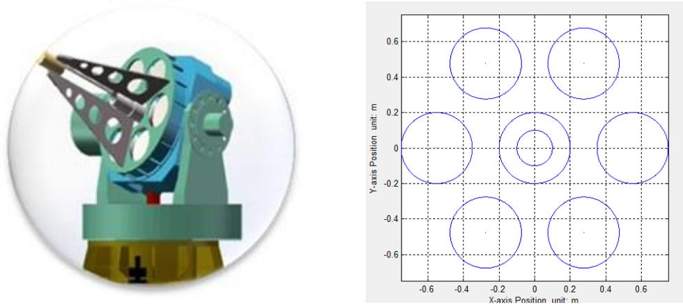
Figure 1. The structure of segmented mirrors telescope (L: concept map; R: array configuration diagram)
