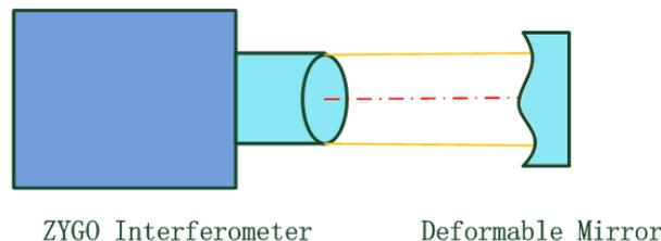
Figure 1 The diagram of measuring setup
