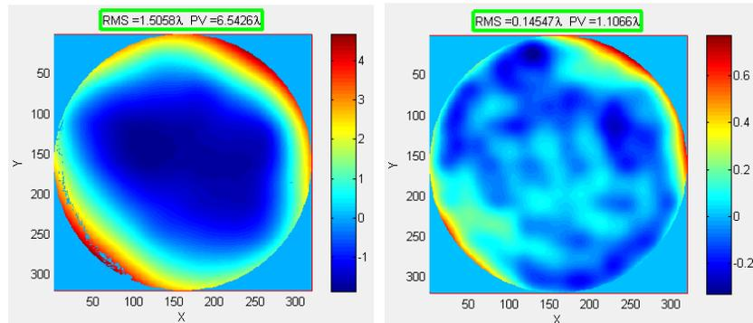
Figure 4 (a)The initial surface of DM; (b)The corrected surface of DM through 25 iterations
