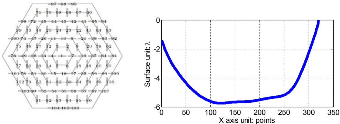
Figure 2 (a)The geometry of the 109-channel DM actuators; (b)The cross section of initial DM surface with all zero voltage channels
