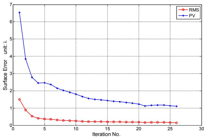
Figure 5 Wavefront phase error of DM correction
