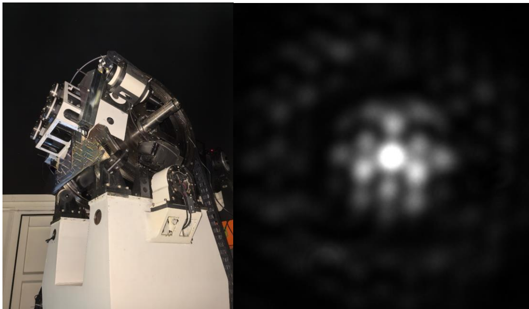
Figure 12 On-site photo of the telescope and far-field image with co-phasing correction
