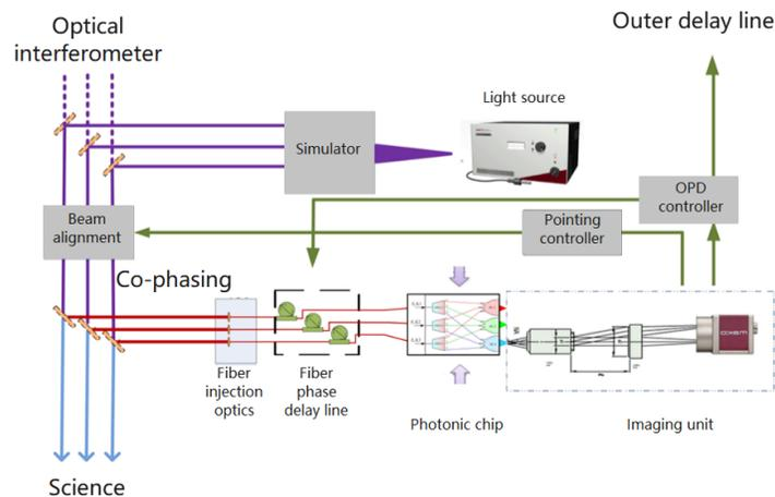
Figure 6. The schematic map of CPD co-phasing experimental set-up
