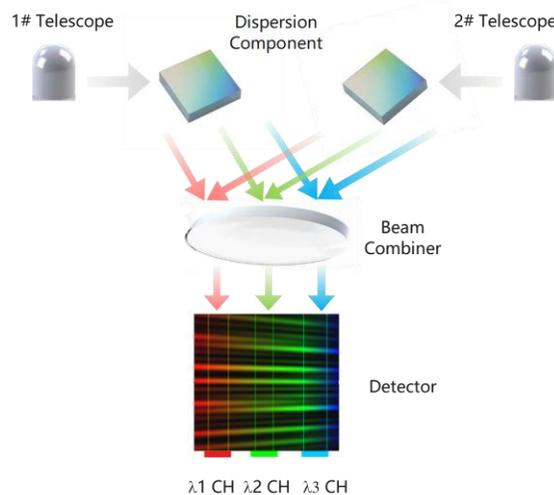
Figure 1. Basic conception of CPD method applied to optical long baseline interferometers
