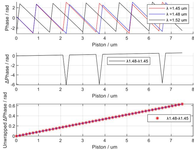
Figure 4. The linear relationship between CPD and OPD utilizing piston sweeping
