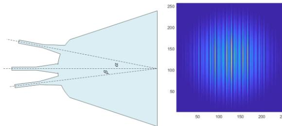
Figure 3. The tapered waveguide structure and simulated fringes captured at the output end of the chip
