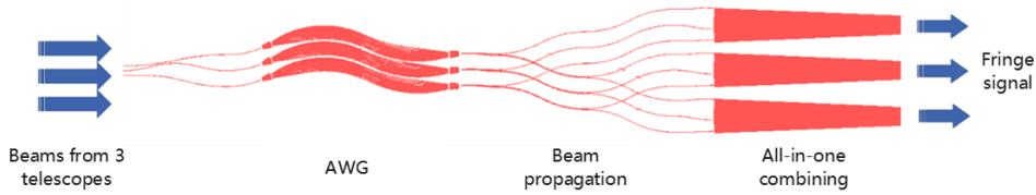
Figure 2. Basic concept of CPD method applied to optical long baseline interferometers
